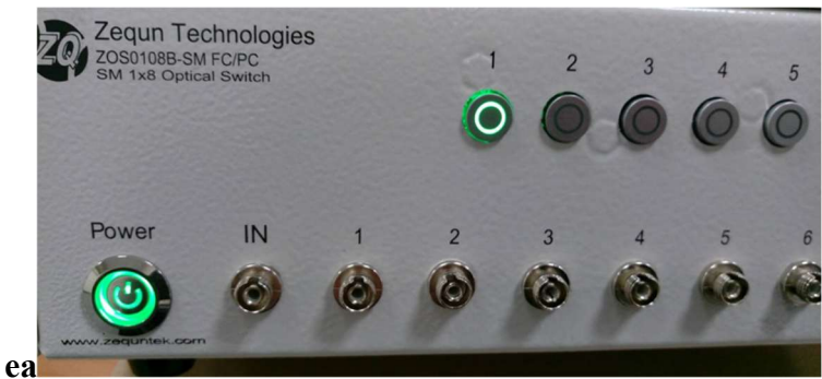
Figure 5.1 LED shows the status of the channel
